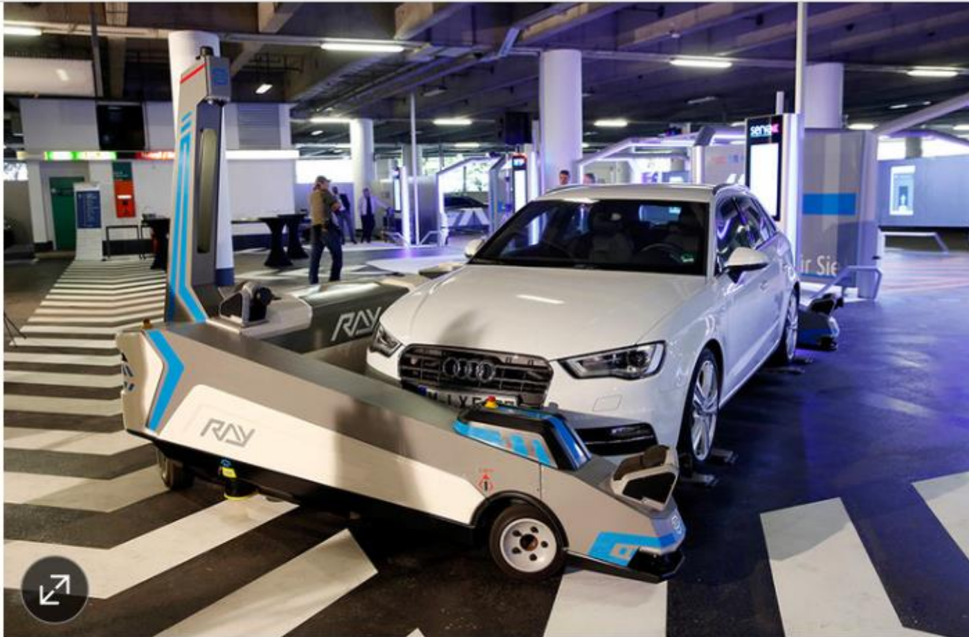
'Ray,' the car-parking robot at the Düsseldorf Airport, in Germany, delivers cars to the curb after passengers land and increased garage capacity by 32%. PHOTO: ANDREAS WIESE
