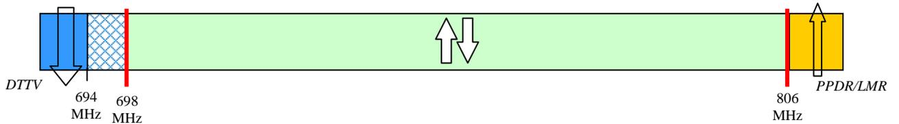
Figure 2. Harmonised all-TDD Arrangement of 698-806 MHz band
