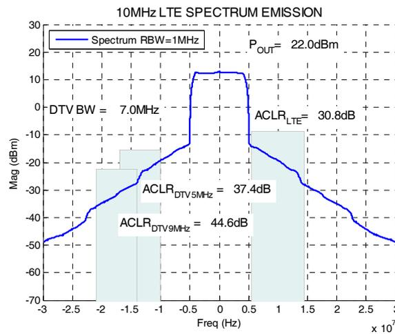
Figure 8. ACLR for full band allocation (5 RBs) to UE
