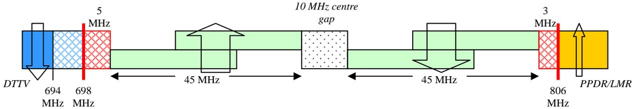
Figure 1. Harmonised FDD Arrangement of 698-806 MHz band
