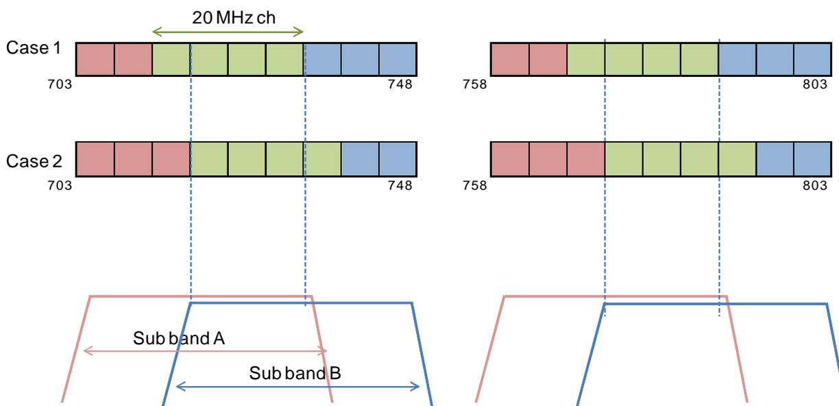
Figure 12. 20 MHz channel positions with 5 MHz raster
