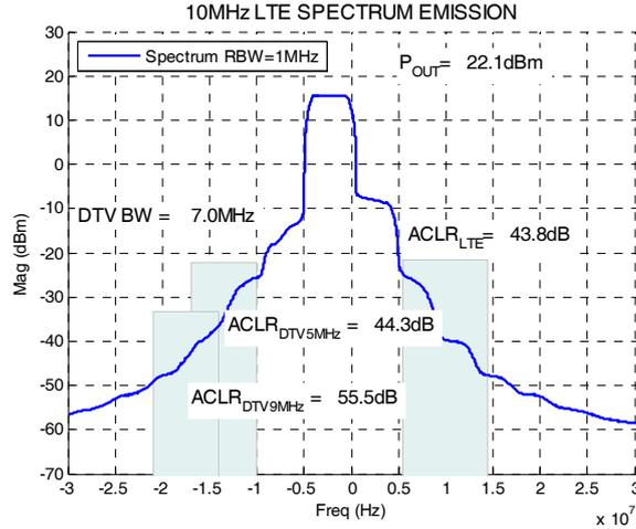
Figure 10. ACLR for partial band allocation (25 RBs, offset 0) to UE
