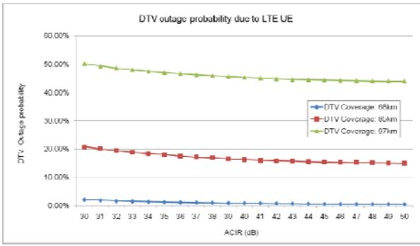
(a) DTV outage probability when LTE UE causes the interference to DTV Rx
