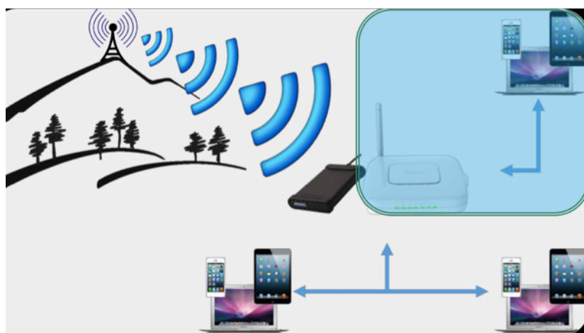
Fig. 8. Near cloud architecture, with small form factor network appliance (blue inset) providing broadband streaming, storage and caching of targeted content in the local "near cloud". This near cloud node is connected through a bandwidth constrained pipe to the internet.
