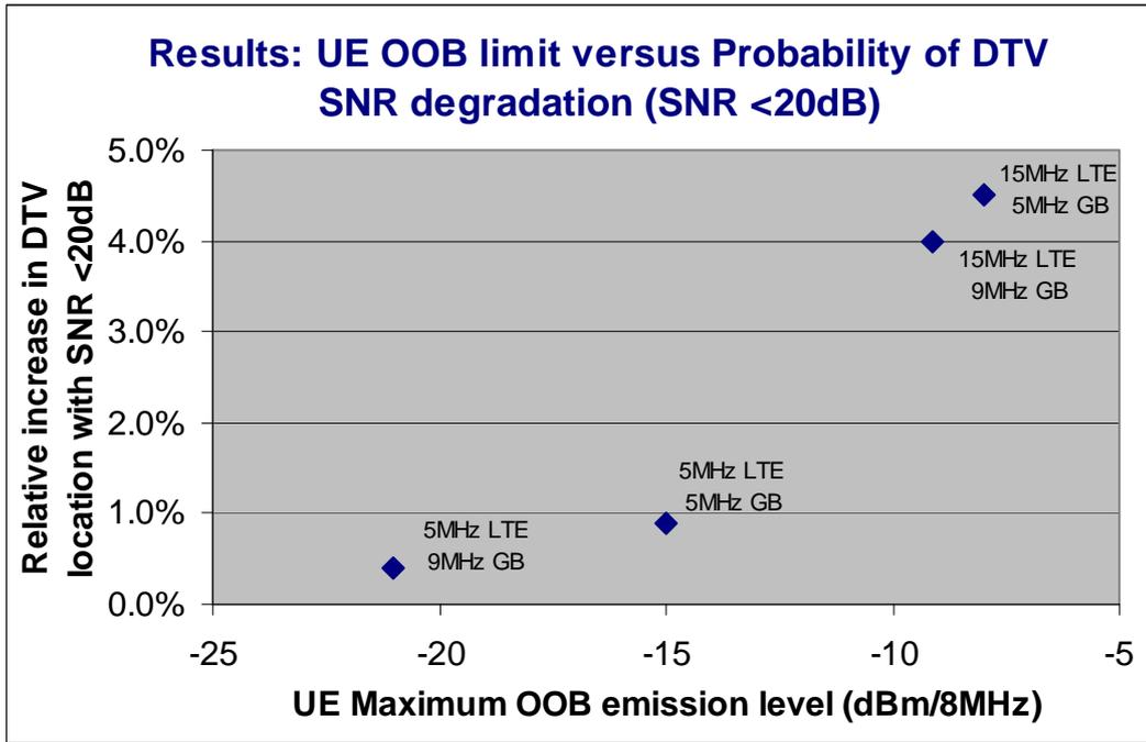
Figure 7. UE OOB limit versus probability of DTV SNR degradation < 20dB
