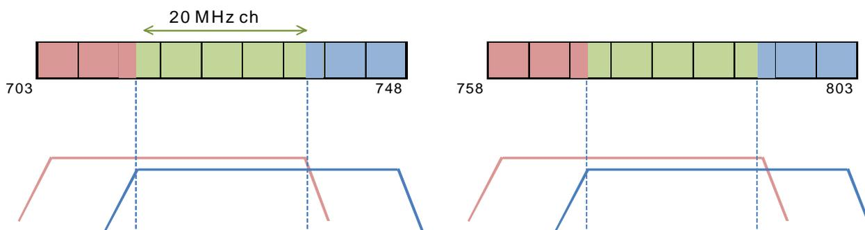
Figure 11. 20 MHz channel in the middle of the band
