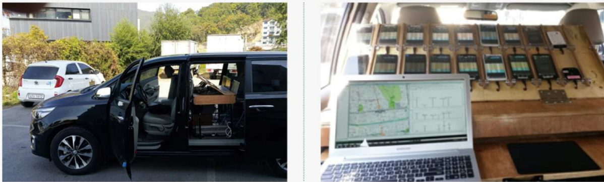
<Figure 24> Drive test vehicle and mobile installation
