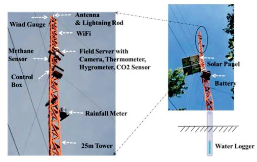
Figure 2-3-4: Tower at Measuring Point A,B and C
