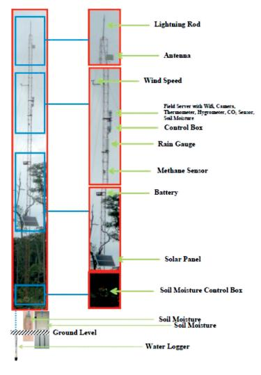
Figure 2-3-5 Tower at Measuring Point D
