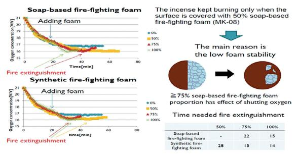
Figure 2-3-9: Performance Evaluation Between Soap and Synthetic Firefighting Foam
