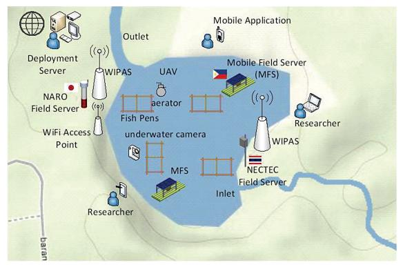
Figure 2-1-4: System configuration in Palapakin lake
