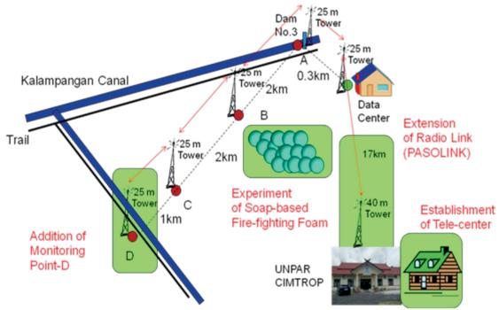
Figure 2-3-3. Network Configuration of Remote Monitoring System
